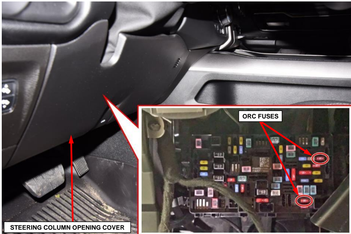
Figure 6 – ORC Fuses F28 and F65
