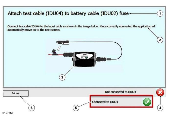
Description Description Item Item Attach test cable (IDU04) to battery cable 2 IDU04 cable connection instructions 1 (IDU02) fuse 3 Cable connection illustration 4 IDU04 not connected icon 5 IDU04 connected icon 6 Exit test button
