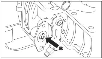
Figure 11 - Spring Brake Installation
