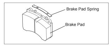
Figure 13 – Pad Retaining Spring Installation
