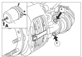
Figure 3 – Actuator Spring Caging and Removal
