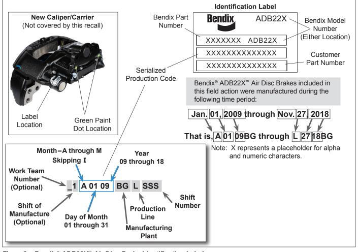
Figure 2 – Bendix® ADB22X™ Air Disc Brake Identification Label
