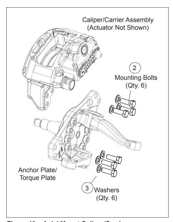
Figure 10 – Axial Mount Caliper/Carrier
