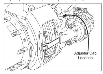
Figure 6 - Adjuster Cap Location
