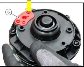
8. Tighten the valve block (6) fastening screws (5) to 0.9 Nm
