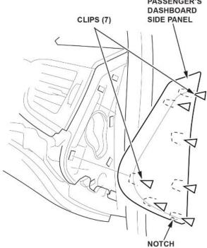
Remove the bolts and screws. SCREWS (5)
