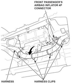
Remove the mounting nuts and mounting bolts from the passenger's front airbag. MOUNTING NUTS
