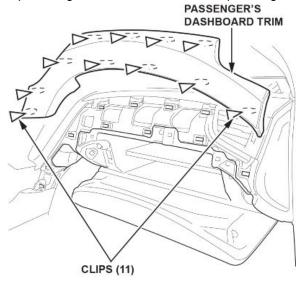
2. Remove the passenger's dashboard side panel. PASSENGER'S DASHBOARD
