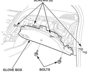
4. Release the hook and pull the glove box out to detach the clip. KEYLESS ACCESS
