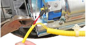
3.2. Strip away about **1 inch** of the red wire insulation, then twist the wires together.
