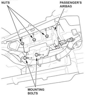
9. Release the pins and remove the passenger's front airbag.
