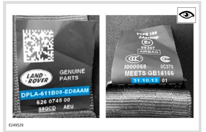
Vehicles with ebony seatbelts only: inspect both sides of the front left seatbelt label for the production date and part number.
