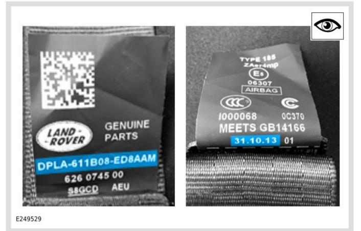
**Vehicles with espresso seatbelts only:** visually inspect both sides of the **front left** seatbelt label for the production date and part number.
