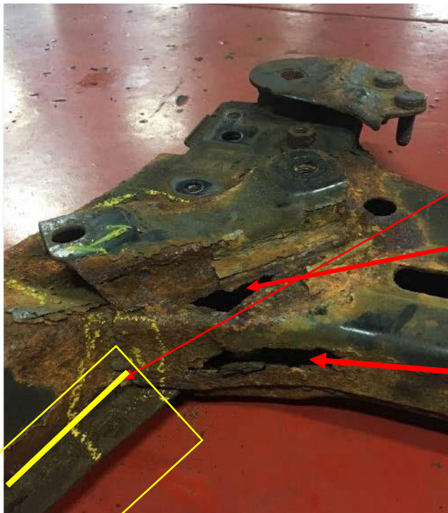
Inside Top View: Damaged Cross member
