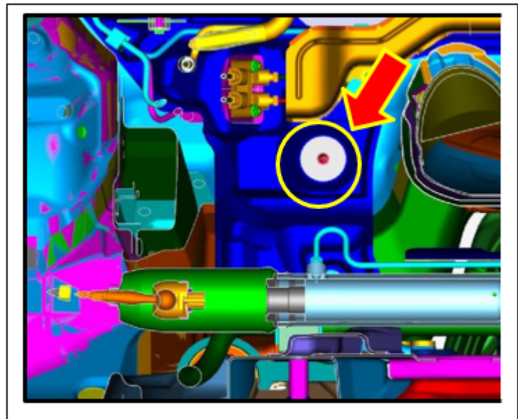
Drain pipe position to insert the drain hose
