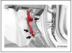
h. Remove the protective tape and connect the connectors to the junction block.
