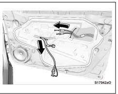
3. REINSTALL THE FRONT DOOR SERVICE HOLE COVER a. Remove the tape that is fastening the upper half of the service hole cover
