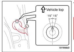
7. CHECK FRONT DOOR GROMMET INSTALATION CONDITIONS
