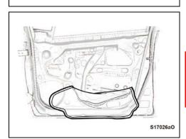
e. Using tape, secure the detached upper half of the service hole cover and place it in a way where it will not interfere with the remaining steps of the repair
