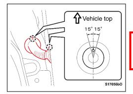
f. Install the front door grommets with the alignment marks at the top (in the range specified in the illustration)
