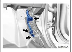
b. Disconnect the connectors from the junction block.
