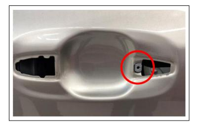
c. Pull the wire harness through the door. It is not necessary to pull the harness through the Apillar.
