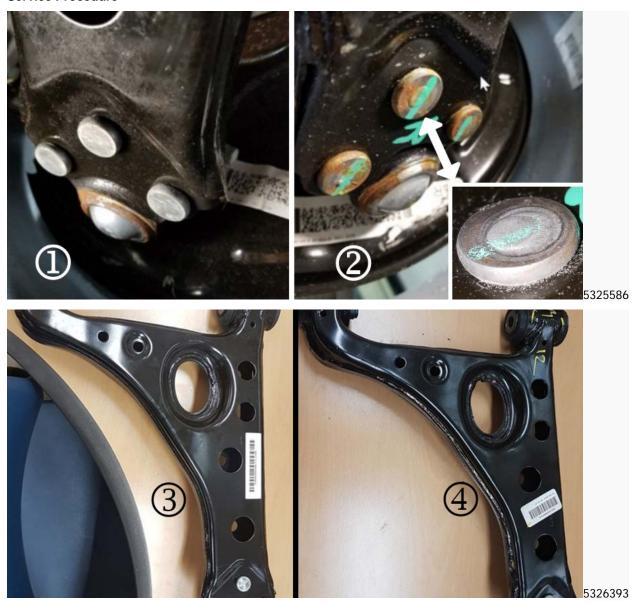
**Note**: Vehicles may or may not have paint marks on the rivets. This is not relevant to the inspection – we are only looking for the circular die mark on the rivets.
