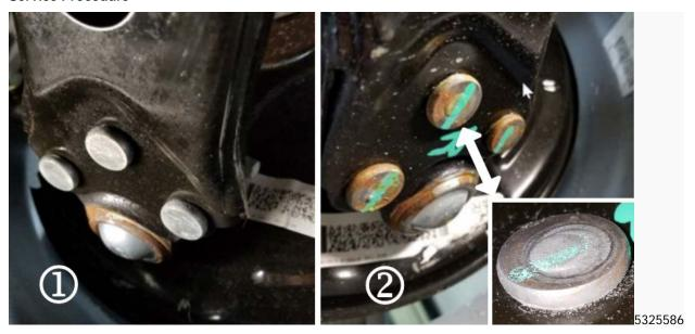
**Note**: Vehicles may or may not have paint marks on the rivets. This is not relevant to the inspection – we are only looking for the circular die mark on the rivets.
