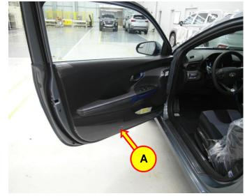
2. Using an automotive trim removal tool, gently pry and remove the front inner door cover (B).
