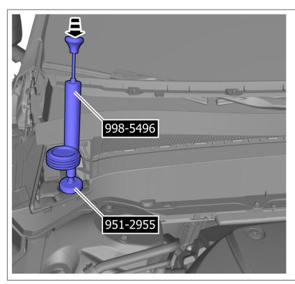
Special Tool: T9985496, ENGINE COOLANT
