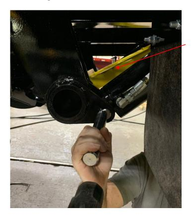
To help with accessibility you may raise the main tail as high as it will go but you must make sure it is properly held up to ensure the tail does not drop while doing service.
