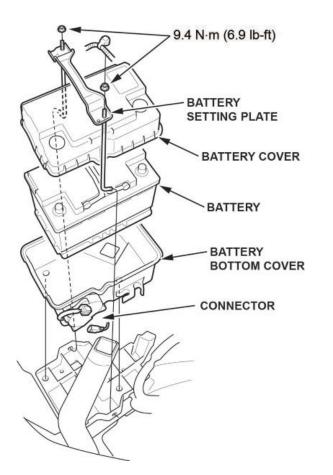
5. Install a new battery. Then reinstall the battery cover, and the setting plate in the reverse order of removal.
