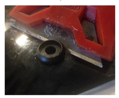
12. Remove the old glue from the mounting holes.
