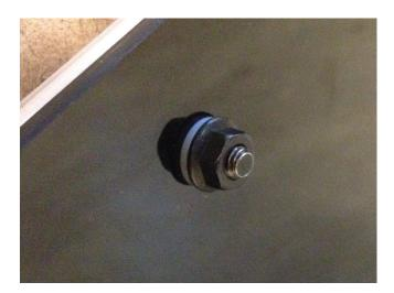
18. Install the two nut caps. Ensure the nut covers are fully seated.
