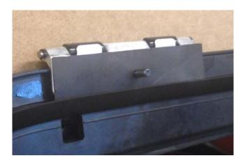
15. Install "E" clips onto the hinge pins.
