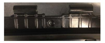
9. Use a putty knife to de-bond the plastic hinge strip from the glass.
