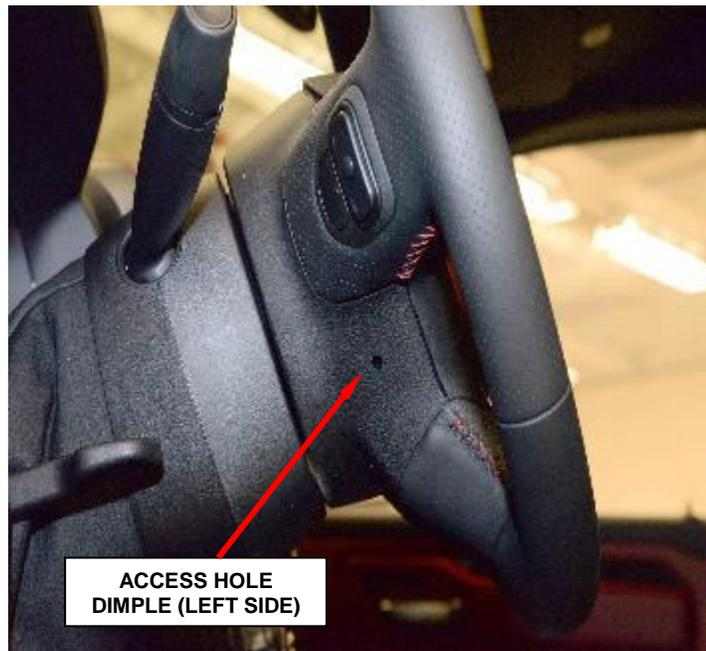
**Figure 1 – Access Hole Dimples (DAB)**
