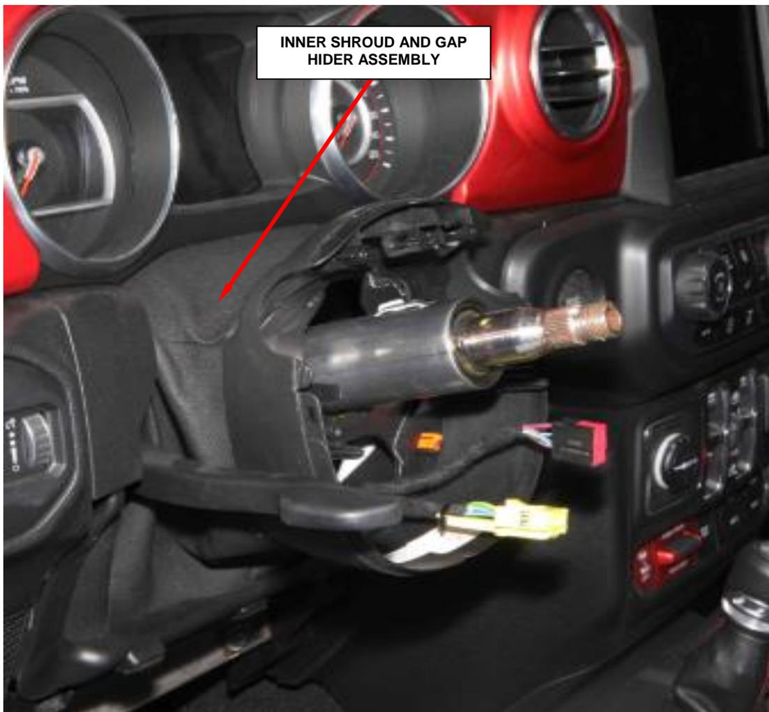
**Figure 27 – Inner Shroud and Gap Hider Assembly**
