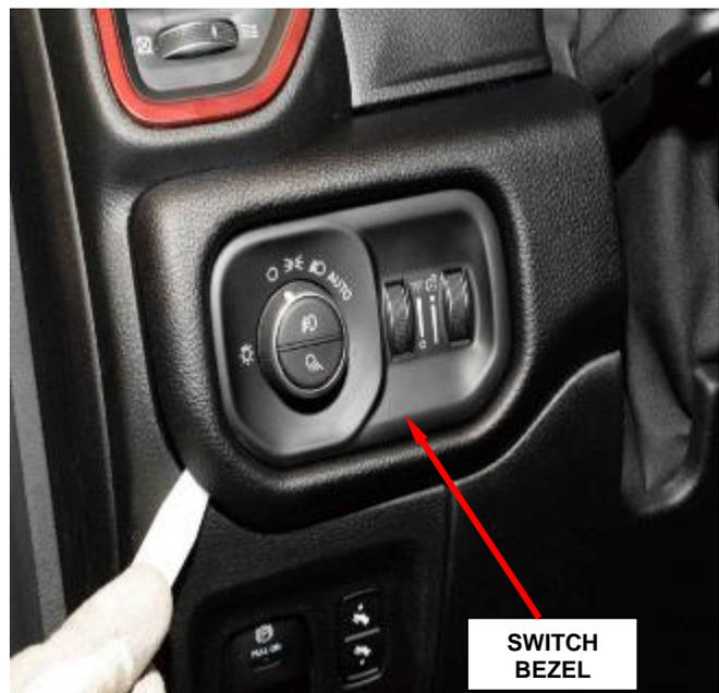
**Figure 11 – Headlamp Switch Bezel**
