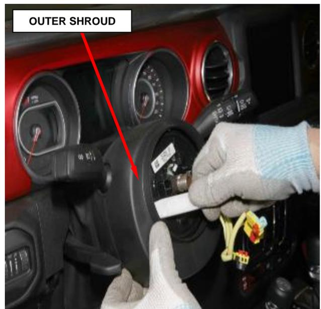
**Figure 24 – Outer Shroud**
