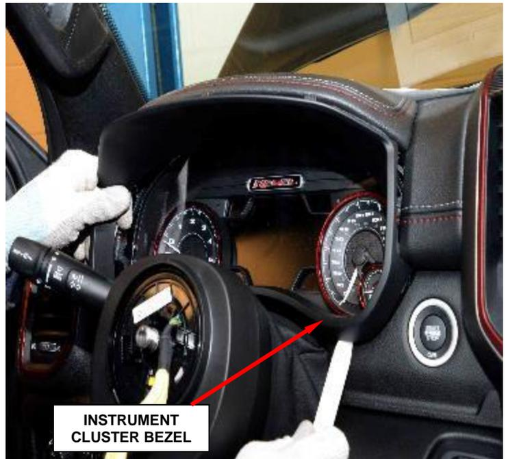
**Figure 8 – Instrument Cluster Bezel**
