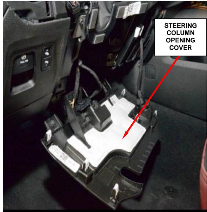
**Figure 12 – Steering Column Opening Cover**
