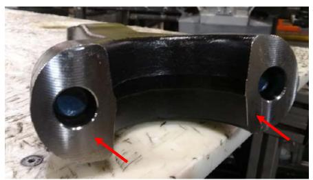
Figure 4 – New (Undamaged) Joint Surface
