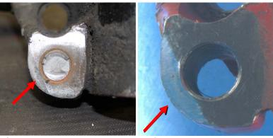
Figure 3 – Dent at the Loose Joint
