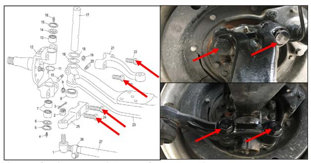
Figure 1 – Steering Arm and Tie Rod Arm Capscrew Location
