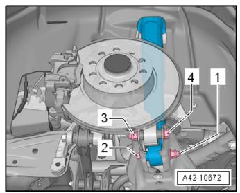
Disconnecting stabilizer link from lower control arm:
