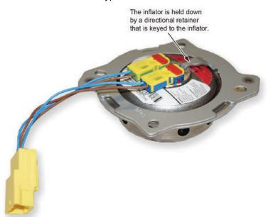
10.3.1. Place the inflator into the opening with the inflator harness toward the bottom of the airbag module. The retainer plate
