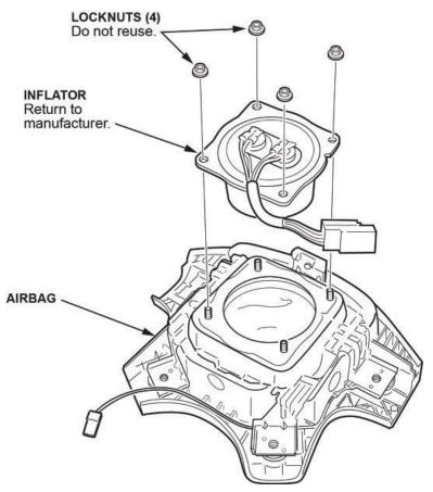
8. Use shop air to clean any debris that may be on the inflator, then remove the inflator from the airbag module.
