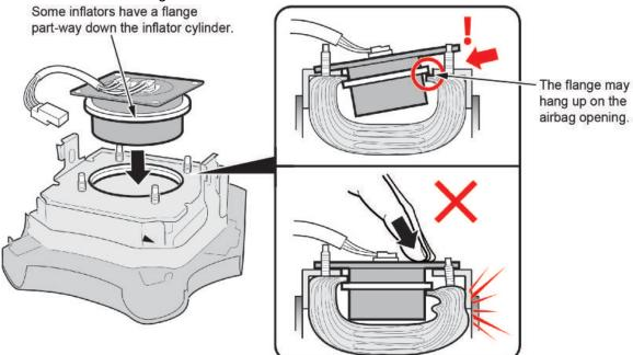
10.2.2. Using a pair of pliers, gently pull up on each stud up while pushing the inflator module down until the airbag is properly seated within the airbag module, then go to step 11.
