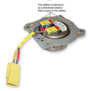
10.4.1. Place the inflator into the opening with the inflator harness toward the bottom of the airbag module.
