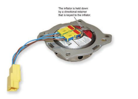
10.2.1. Place the inflator into the opening with the inflator harness toward the bottom of the airbag.
