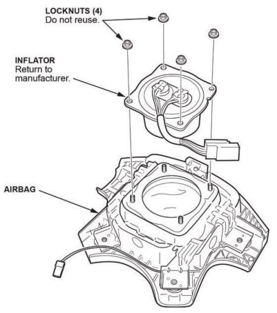
8. Use shop air to clean any debris that may be on the inflator, then remove the inflator from the airbag.
