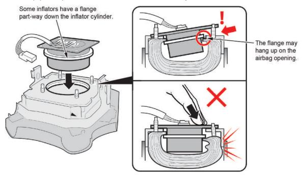
10.1.2. Using a pair of pliers, gently pull up on each stud up while pushing the inflator module down until the airbag is properly seated within the airbag module.
