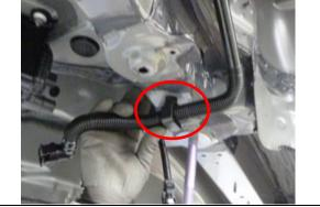
d) Secure clip to underside of body.
