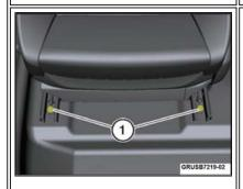
Check if the torque of both front bolts (1) are correct,
