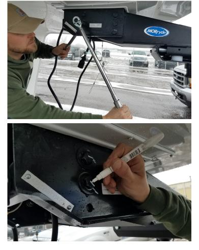
**Step 3:** Use a paint marker and torque mark all bolts.
