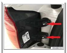
2. **Before** removing the tail light mounting nuts, carefully inspect the tail light mounting areas shown to the left for signs of cracking.
