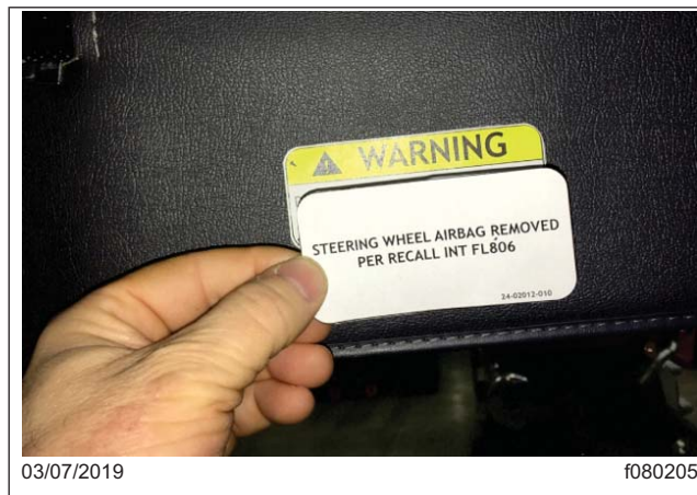
Fig. 13, Installing the Stickers on the Sun Visor
