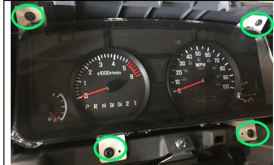
Figure 5 – Remove Torx® Bolts
