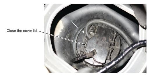
14. Install the fuel tank access panel and rear seat.
