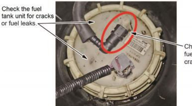
Check around the fuel feed port for cracks or fuel leaks.
