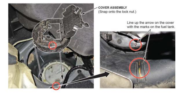
9. Connect the fuel line and the connector as shown.
