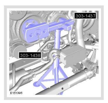
Use a suitable vehicle stand to support the special tools 303-1437 and 303-1438.
