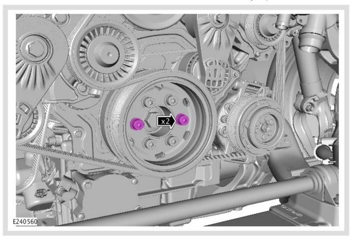
Install the original outer crankshaft pulley bolt(s).
