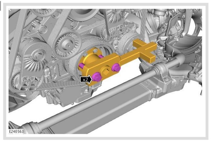
Remove the 2 outer crankshaft pulley bolt(s) from special tool 303-1437.
