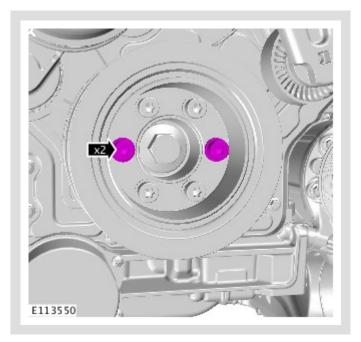
Remove and set to the side only the 2 highlighted outer crankshaft pulley bolt(s).
