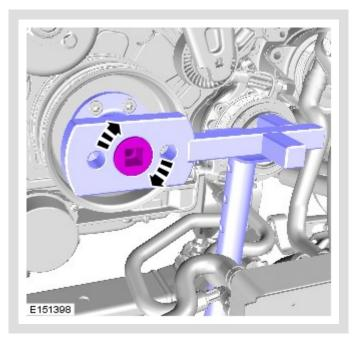
Remove the center main crankshaft pulley bolt(s).
