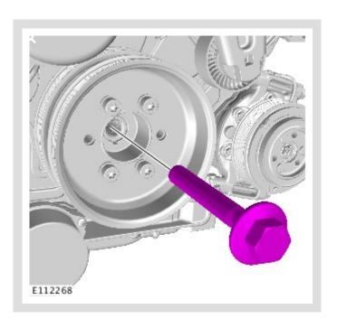
Remove and discard the center main crankshaft pulley bolt(s).
