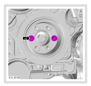
Install the 2 original outer crankshaft pulley bolt(s).
