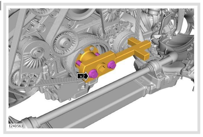
Using the bolt(s) for special tool 303-1437, install the 2 bolt(s) to the crankshaft pulley.
