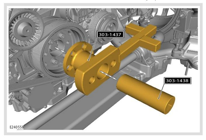
Remove the vehicle stand and special tools 303-1437 and 303-1438.
