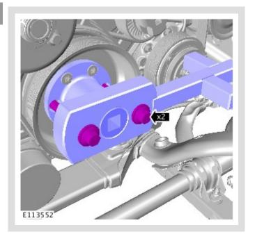
Using the bolt(s) for special tool 303-1437, install the 2 bolt(s) to the crankshaft pulley.
