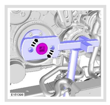
Remove the center main crankshaft pulley bolt(s).
