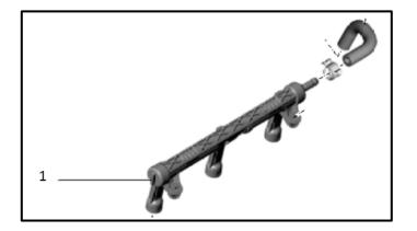
Replace left and right low pressure fuel rails <1>.
