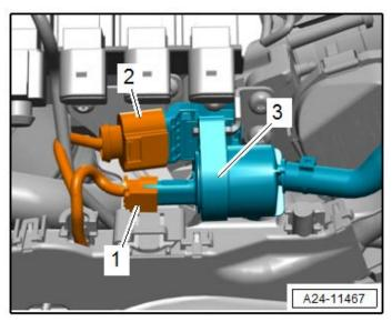
Release the catches <arrow> and push the wiring duct <1> to the rear.
