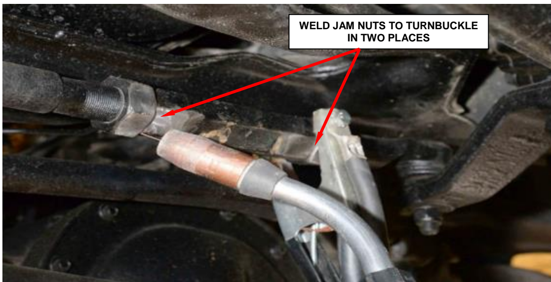
Figure 9 – Weld Both Jam Nuts to the Turnbuckle
