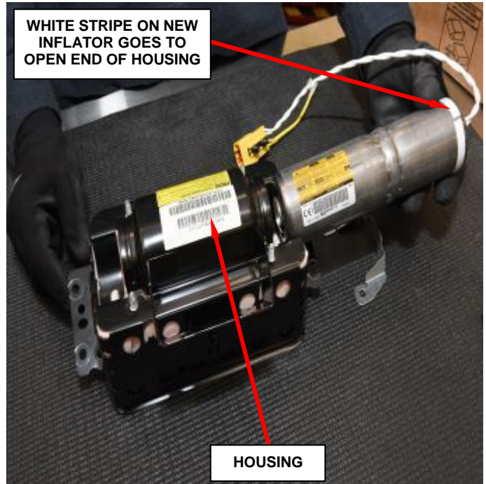
Figure 43 – Install New Inflator to Housing
