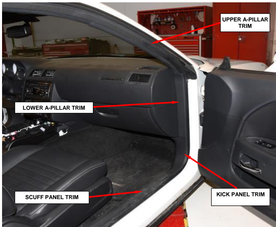
Figure 32 – Door Opening Trim (Right Side Shown, Left Side Similar)
