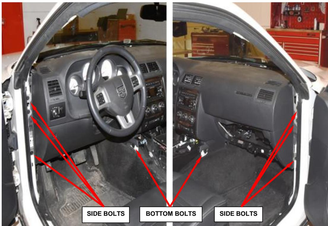
**Figure 47 – Side and Bottom Retaining Bolts**
