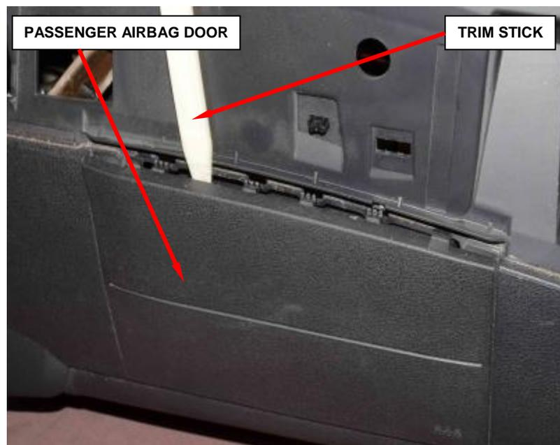
**Figure 83 – Passenger Airbag Door**
