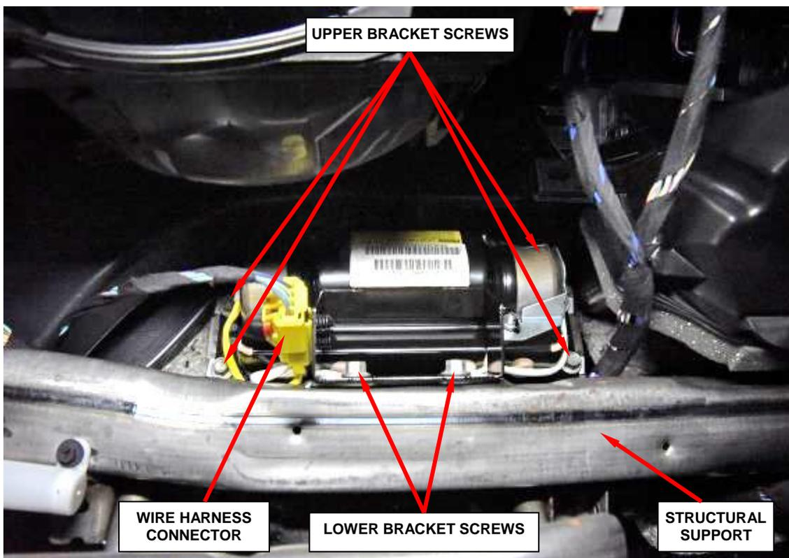
**Figure 45 – PAB Housing, Inflator and Cushion to be Removed a Unit
