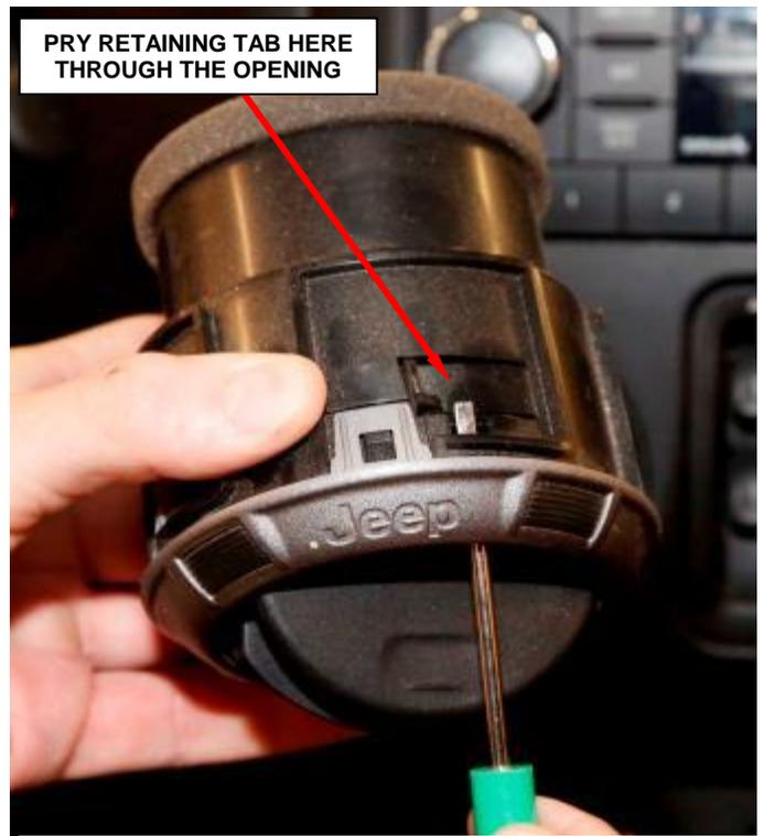
**Figure 95 - HVAC Outlet Tab**
