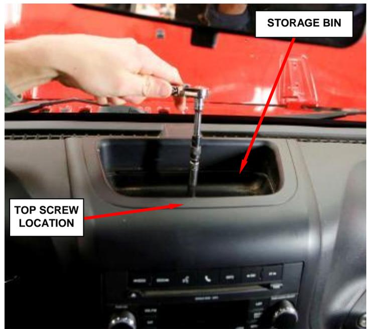
Figure 97 – Center Bezel Screws
