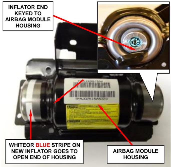
**Figure 37 – Install New Inflator to Housing**
