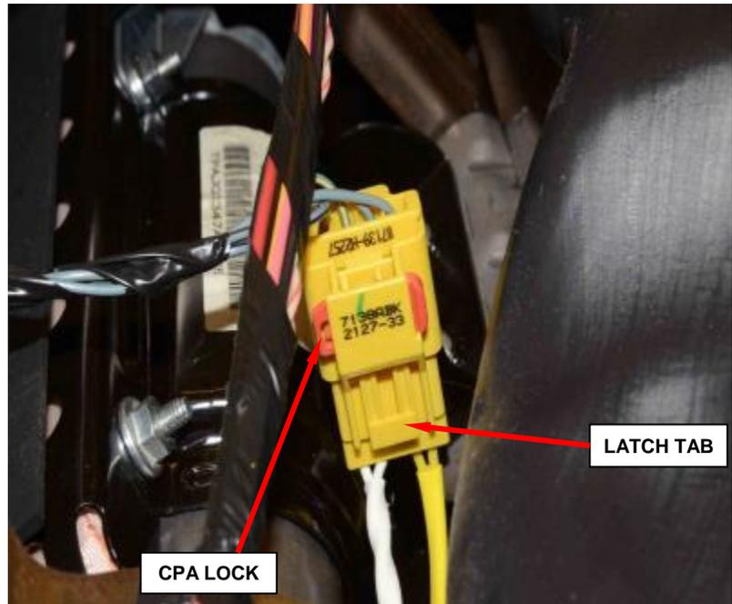
**Figure 82 - Airbag Inflator Pigtail Connector**
