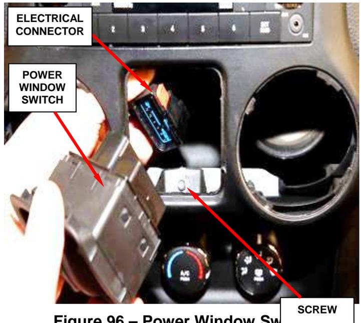
Figure 96 – Power Window Switch
