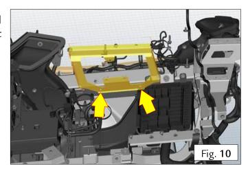
2.9. Install the new airbag reinforcement bracket code 745714 using the Raymond brackets code 67278400. Tight the indicated screws to the torque of 5 Nm Class B- Fig. 11.
