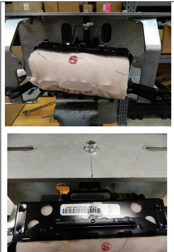
g) Mount the airbag into the mounting bracket as shown. Pass the stud on the adaptor through the hole in the middle of the bracket with the nut.
