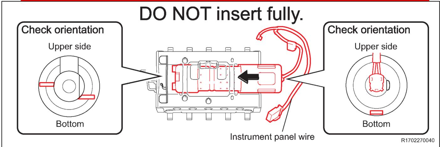
b) Connect the connector to the inflator and ensure that the connector lock is fully engaged as shown.
