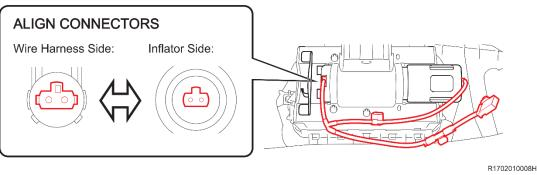
a) Fully insert the inflator and ensure that the inflator is correctly orented as shown. NOTE: DO NOT pinch the wiring between the bracket and the inflator.
