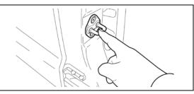
If the anti-static kit is not available, before starting work and periodically while working on the vehicle, touch a metallic part of the vehicle to discharge static electricity in the body.
