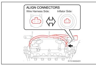
Connect the connector and the secondary lock
