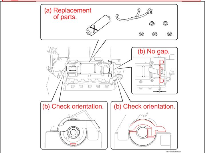
j) Tighten the 5 nuts evenly in several increments in the sequence shown. Use a socket driver or torque wrench to tighten the nuts.
