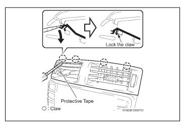
Removing the No. 3 air register
