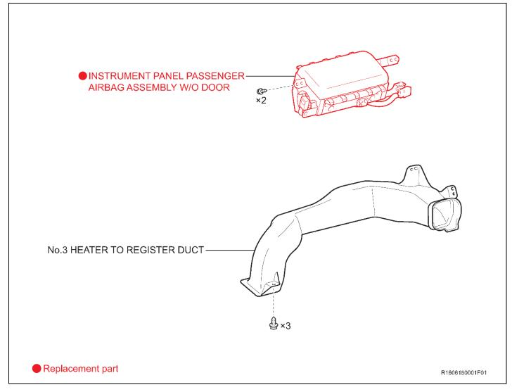
c) Remove the 4 bolts, disengage the straps, and then remove the airbag assembly. NOTE: Use a screwdriver with the tip wrapped in tape to remove the airbag from the dash.
