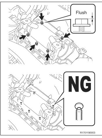
b) Mount the adaptors (579943-3R3) to the airbag as shown.NOTE: The 6mm stud mounts to the airbag.
