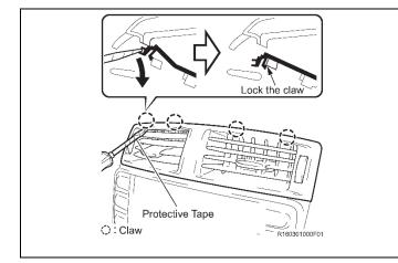
Removing the No. 3 air register
