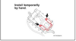
e) Temporarily install a **NEW** plate and airbag inflator with the 2 **NEW** self-locking nuts.
