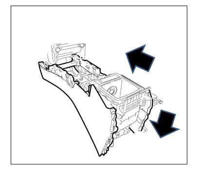
a) Install the front of the console box with rear section lifted as shown.
