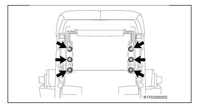
c) Reengage the 6 claws on each side of the console as shown.
