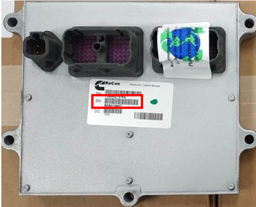
Figure 1 - Location of ECM Serial Number
