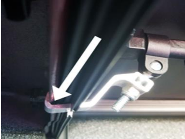
Correct installation of bracket clamp hook
