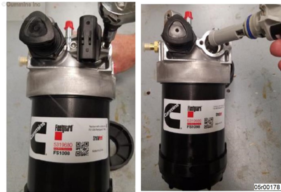
Figure 5, Removal of Heating Element.
