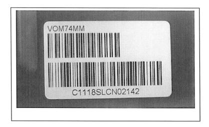
The alphanumeric serial code at the bottom of the label can be used to identify the affected items. As an Example (C1118SLCN02142) the first letter is the revision "C." The following four numbers are a date code in MMYY format. The affected products will have serial number starting with A, B, or C.
