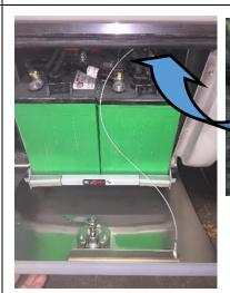
Use the 5/16" socket/nut driver to remove the tek screw from the inside floor aluminum rail.
