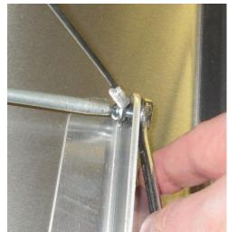
Hold the machine screw of the cable with the screwdriver while loosening the nut on the other side with the 9mm wrench.
