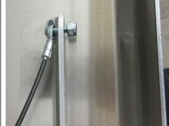
Install the other loop of the insulated cable with the machine screw, washer, and cable loop on the bottom of the door latch and the self locking nut on the top. Tighten nut on the
