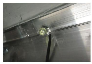
Install the new insulated cable fastening one cable loop to the aluminum floor rail with the 5/16" tek screw back into the same hole.
