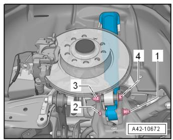
Disconnecting stabilizer link from lower control arm:
