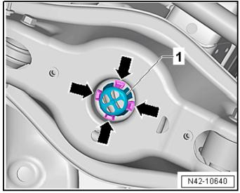
Disconnect level control system sensor (if equipped):
