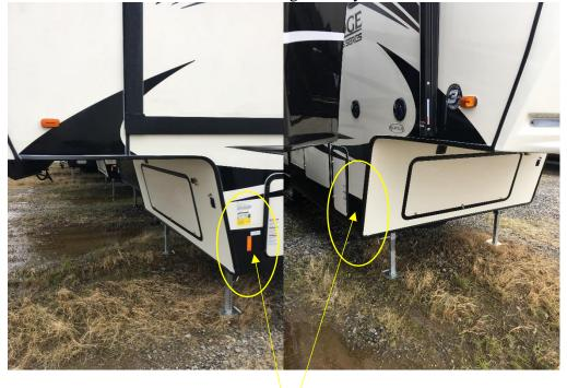
2. Where to install the reflector that is being sent to you.
